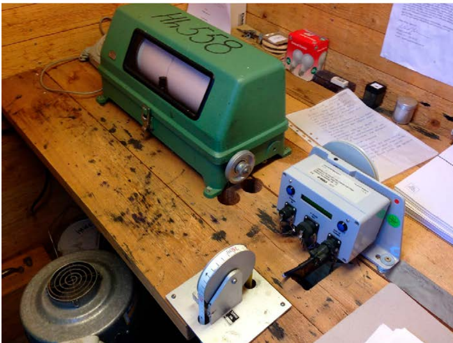
Figure A7-3. The SMHI sea-level gauge, located in a small building in the SFR harbour (photographer: Kent Werner). The upper picture shows the SKB sea-level gauge PFM010038 to the right, consisting of a pressure sensor lowered through a hole in the concrete floor.
