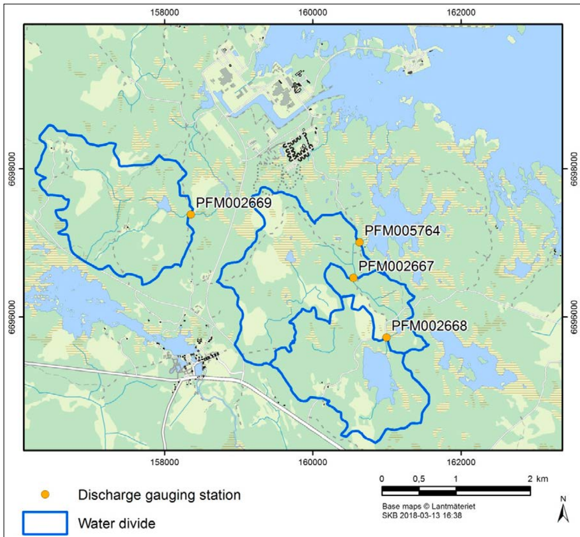
Figure 1-1. Locations and associated catchment areas of the four stream-gauging stations. The PFM005764 catchment area includes the PFM002667 catchment area, which in turn includes the PFM002668 catchment area.
